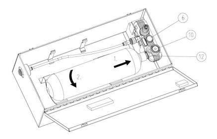
The pressure gauge (10.) on the fitting for the compressed air cartridge now shows the pressure currently prevailing in the cartridge. The pressure equipment is ready for operation when the pointer of the pressure gauge (10.) is in the green part of the scale.
